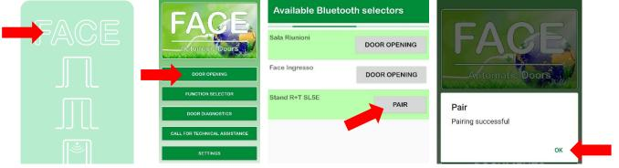
Note: if the Bluetooth connection does not work, deactivate the Bluetooth of your smartphone for a few seconds and reactivate it.
