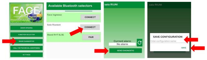
Note: it is possible to connect to the DOOR one smartphone at a time.
