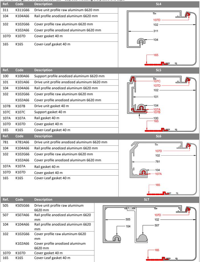
All the aluminium profiles and gaskets needed for the realization of the telescopic automations must be cut 6 mm shorter than the maximum length of the automation (Ld - 6), also including the end caps.
