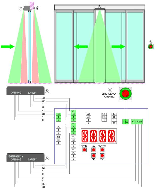
Connect the sensor A side, using the supplied cable to the terminals of the electronic control, as follows:
