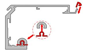
5.4 Secure by front hooking the drive unit on the drive unit profile, placed at a maximum B (as shown in Chapter 4), and secure it with the screws (Note: if there is space, it's better to reduce measure B few centimetres).
