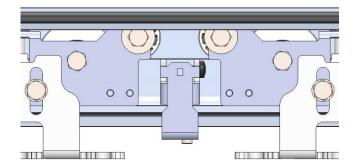
5.8 Insert the belt in the pulley motor drive unit, slide it and pass it around the transmission unit and fix to carriage with the proper springs (see the belt attack position, as shown in Chapter 4).
