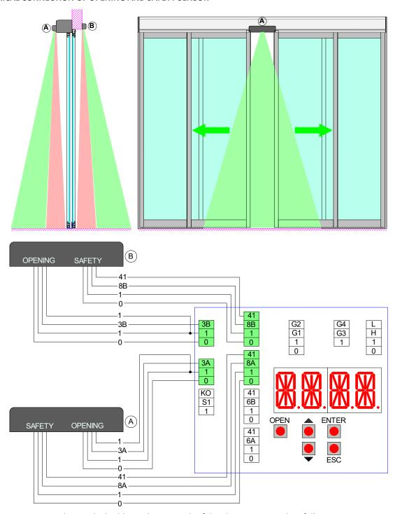
Connect the sensor, using the supplied cable, to the terminals of the electronic control, as follows:
