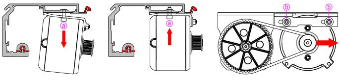
5.5 Secure by front hooking the transmission unit on the drive unit profile, place it to maximum A (as described in Chapter 4), and secure it with the screws.
