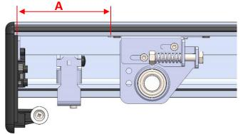
5.6 Insert the carriages in front on the drive unit profile.
