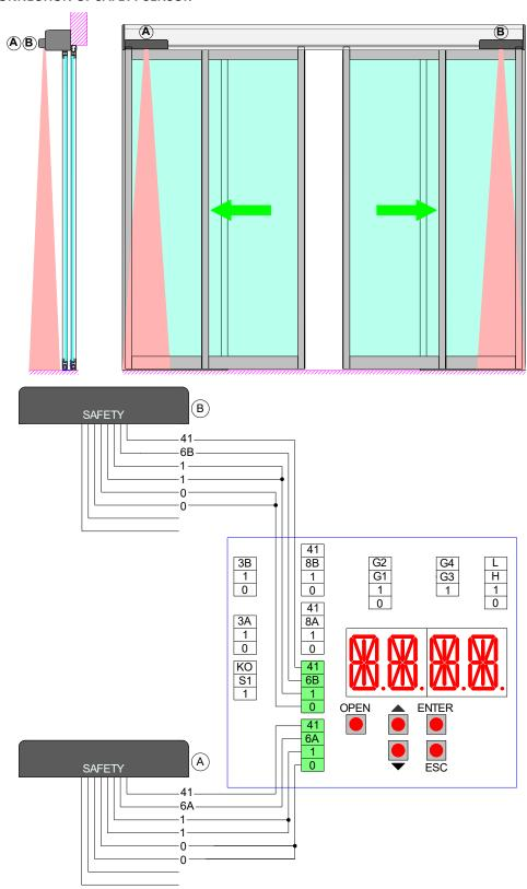
Connect the sensor, using the supplied cable to the terminals of the electronic control as follows:
